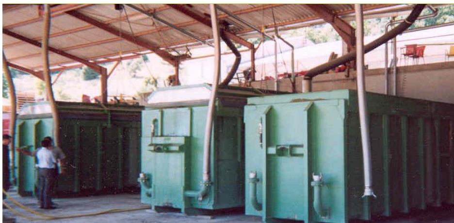
Figure 6 Steam distillation of herbs in Italy (source: Primavera)
