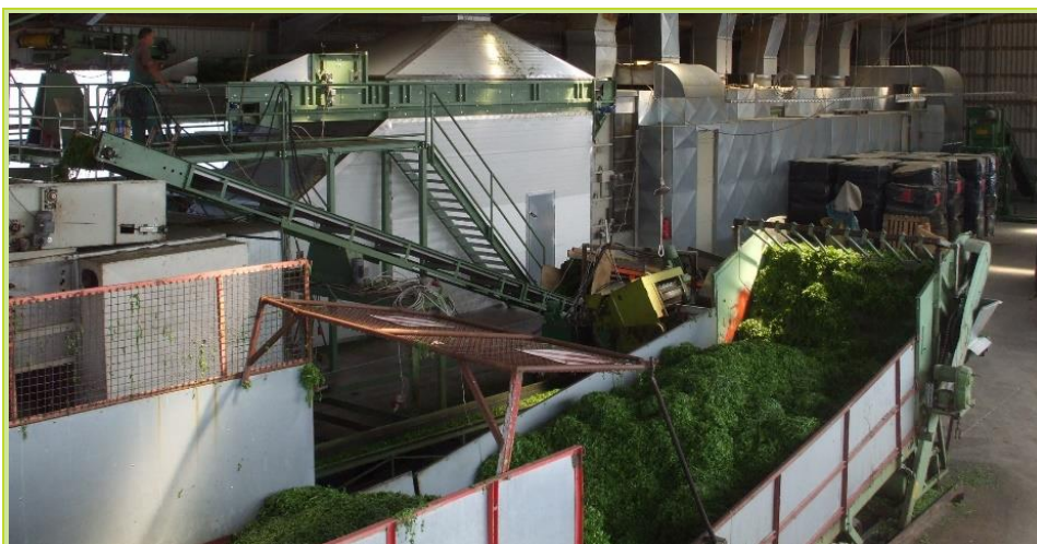
Figure 5 Conveyor-belt dryer of herbs in Germany (source: Argyropoulos & Müller)
